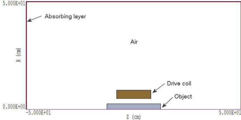
Figure 28: Geometry of example MAGNEAR, dimensions in cm.
