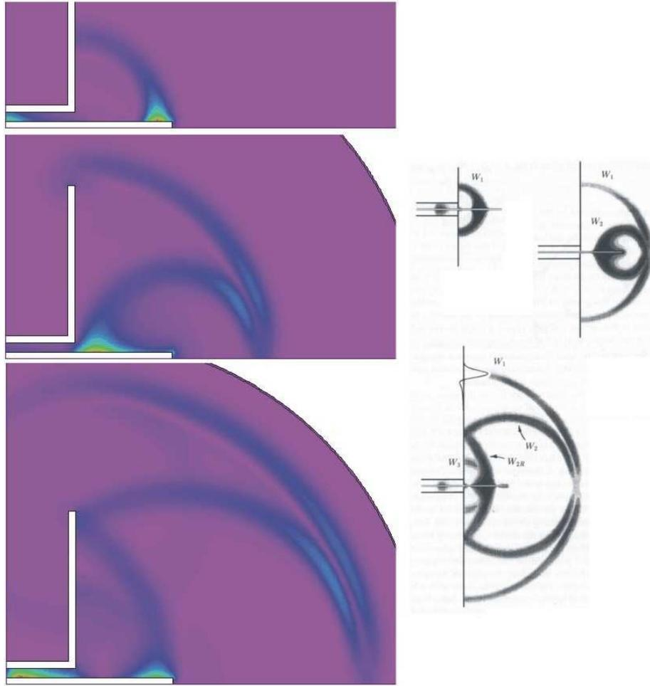
Figure 2: Benchmark test – radiation from a pulsed dipole antenna. Left: **EMP** results,  $r$ - $z$  plots of  $|\mathbf{E}|$  at 1 ns intervals. Right: cross-section plots of  $|\mathbf{E}|$  from J.G. Maloney, G.S. Smith and W.R. Scott, IEEE Trans. Antennas Propagation **AP-38**, 1059 (1990)
