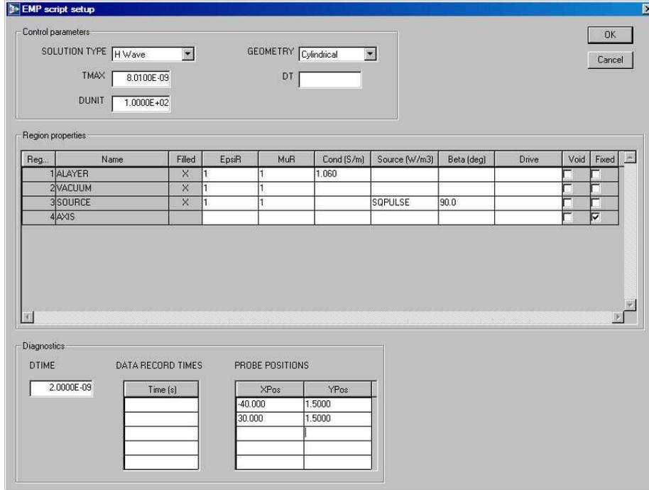
Figure 10: Dialog to set **EMP** control parameters and region properties.
