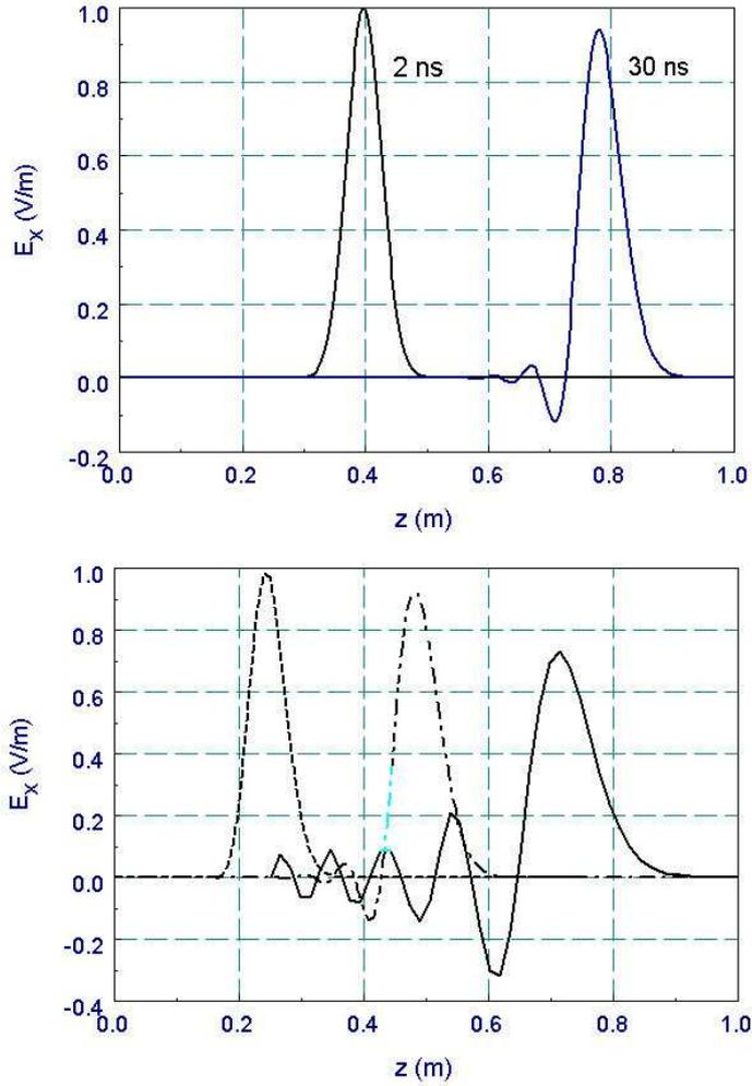
Figure 5: Numerical dispersion in time-domain electromagnetic solution. Gaussian pulse in vacuum, FWHM = 0.067 m. Top: Pulse shapes after 0.6 and 9.0 m propagation for an element width of 0.004 m. Bottom: Pulse shapes after 2.5 m of propagation as a function of element width. Ratio of pulse width to element width: 16.6 (dotted), 8.3 (dashed) and 4.2 (solid).
