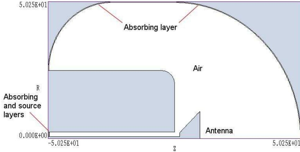
Figure 9: Geometry for the **CONICAL** example. A pulse on a transmission line in a finite-width ground plane drives a conical antenna. Dimensions in cm.
