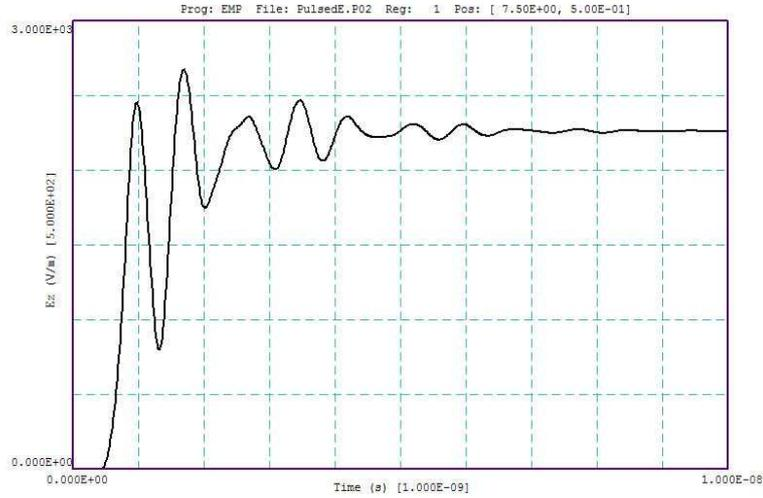
Figure 26: PULSEDE example: calculation of  $E_z(t)$  at  $z = 7.5$  mm,  $r = 0.5$  mm.
