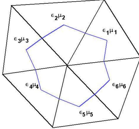
Figure 4: Line integral path through elements surrounding a node.
